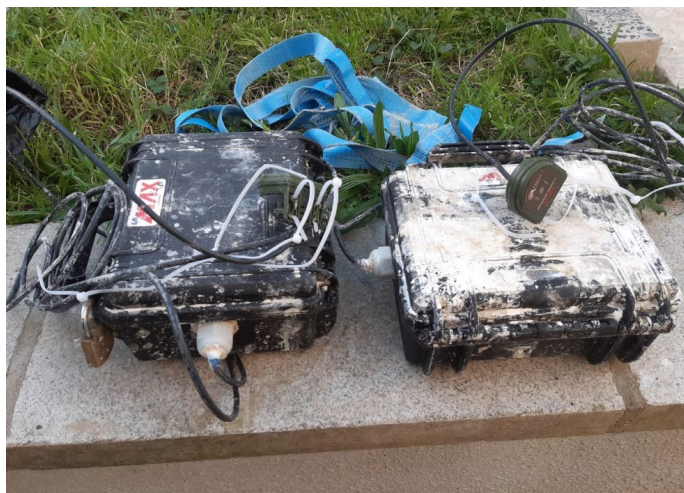
Figure 3.1 Equipment in returned state. The armoured boxes were heavily fouled by bird guano.
