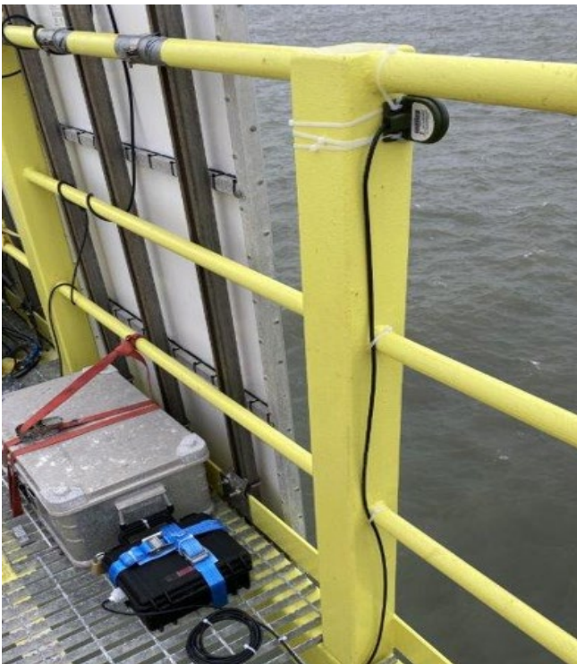
Figure 2.3 Photograph to illustrate the placement of the bat detector on the platform
